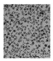
Five-fold twinned, starfish-like Rh nanocrystals consisting of five arms (see TEM) have been synthesized in high yields with the use of [{(CF<sub>3</sub>COO)<sub>2</sub>Rh}<sub>2</sub>] as a precursor to completely eliminate oxidative etching from this system. The as-prepared Rh nanocrystals were shown with great performance as a substrate for SERS.
