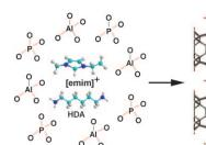
Open for business: The first aluminophosphate molecular sieve with 20-ring pore openings has been synthesized ionothermally using a co-structure-directing agent (see figure; H white, C turquoise, N blue). The new material has a -CLO framework and excellent stability in comparison to the GaPO<sub>4</sub> analogue cloverite. These characteristics indicate its potential applications in separation, catalysis, and gas storage.
