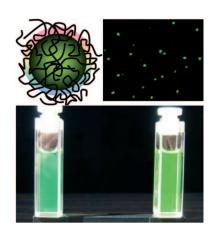
Quantum of solace: Fluorescent carbon dots (surface-passivated carbon nanoparticles) are developed as an alternative to classical semiconductor quantum dots. Gel column chromatography afforded carbon dots with emission yields close to 60%. Their optical properties resemble band-gap transitions found in nanoscale semiconductors, thus suggesting that nanoscale carbon particles acquire essentially semiconductorlike character-
